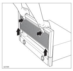
■ Hold the grease filter firmly, and pull it out with the deflector plate as shown.
